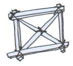
(Cross Beams) By assembling a X in the center of a square you equalize the distances between the opposite corners, creating a ridged shape which Is able to transfer force/mass to the opposite side of the structure
